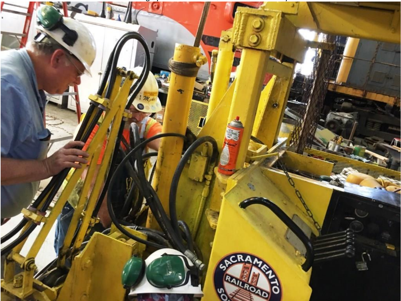
Chris and Mike F. work with Joe on installing the lift cylinder
